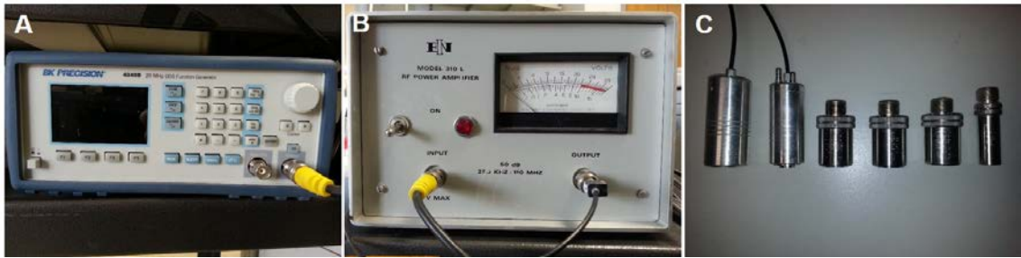
Figure 3.1 Configuration of ultrasound therapy system. (A) Versatile sweep function generator produces either continuous or pulsed waveforms. (B) Generated signal waves are amplified by a radio frequency power amplifier. (C) Various sizes, types and frequencies of ultrasonic transducers. Generated and amplified electrical signal waves are converted into mechanical ultrasound waves by ultrasonic transducers.
