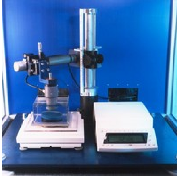
Figure 3.2. Ultrasound power measurement by a radiation force balance. An acoustic absorber placed on the balance absorbs almost 100% of ultrasound waves and the balance measures the weight caused by ultrasound power. http://www.npl.co.uk/
